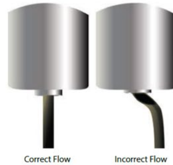
Figure 48. Correct vs incorrect (deflected) flow
